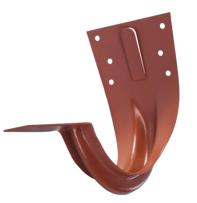
The various gutter brackets must comply with EN 1462 ("Brackets for eaves gutters") standard. The gutter hook should be mounted on the eave plank or at the end of the rafters/counter battens, while the eave board bracket should be attached to a fascia board with an appropriate. Corrosion-resistant screws or nails are usually used for fastening.
