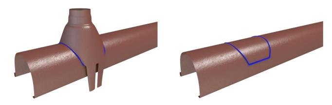
It is advisable to start the cutting with a hacksaw and then expand it into a circular shape with sheet metal scissors. The cutting edge should be at max. 3 cm from the marking. Do not use an angle grinder for cutting, as this will heat up the duct material or hot bouncing particles will damage the coating.
