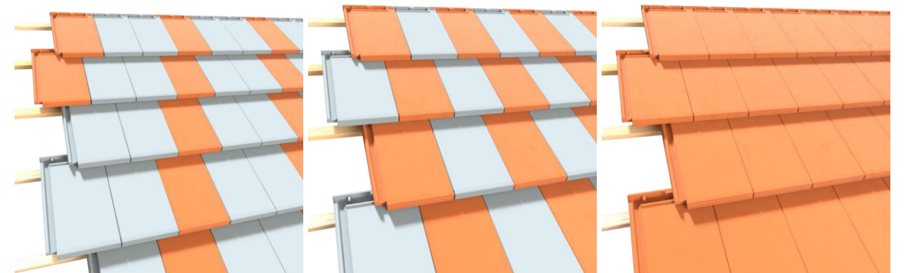
Schema 1:3, schema 1:2 and schema 1:1, with clay interlocking roof tiles installed in bonding
