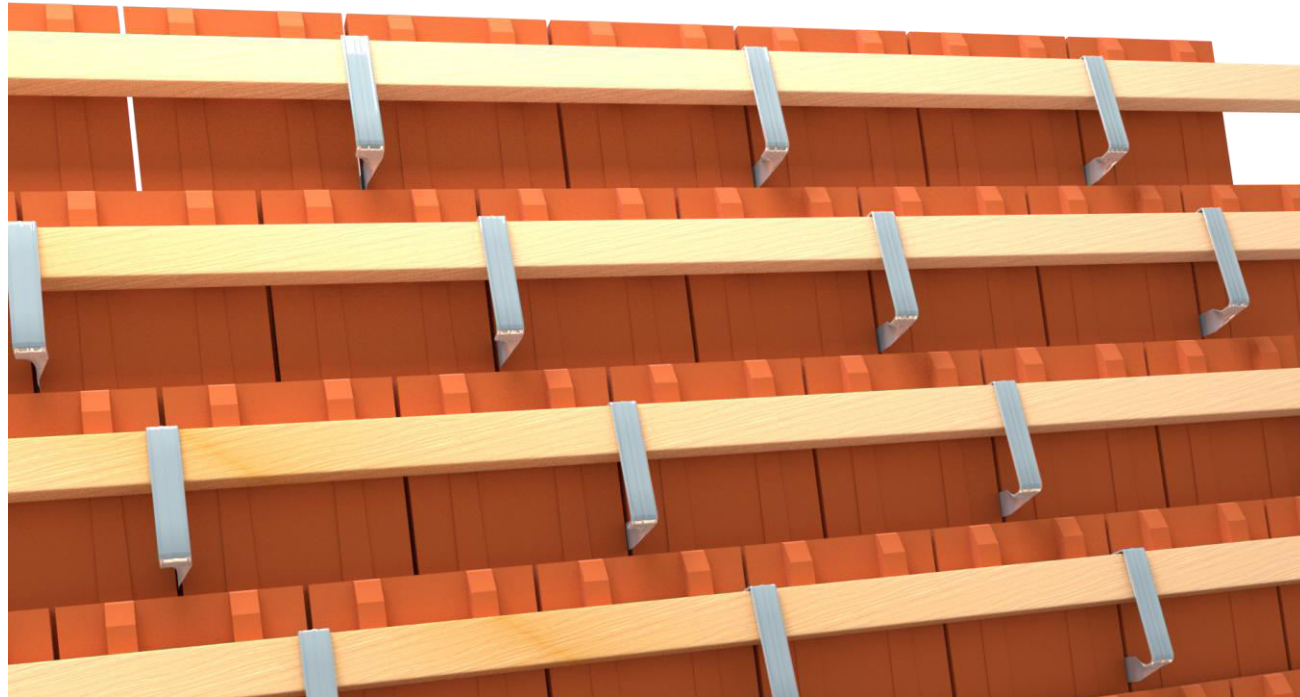
Schema 1:2 with mount-on stormclips, for double cover plain tiles installed in bonding
