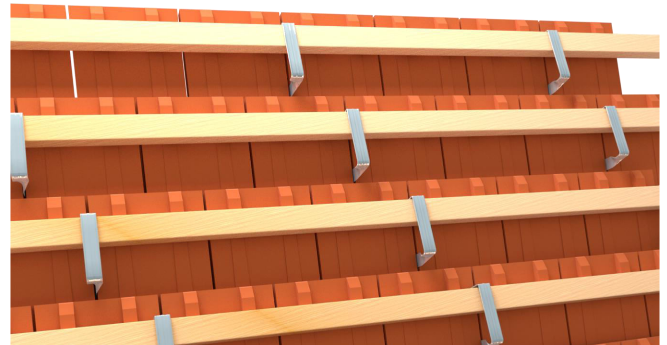
Schema 1:3 with mount-on stormclips, for double cover plain tiles installed in bonding
